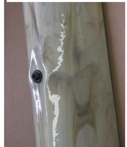
Glass sconce body with central stud protruding, before hemispherical nut is attached.
